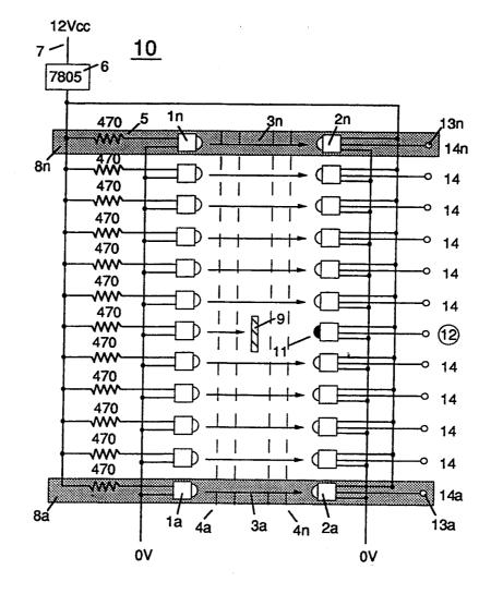
FIGURE 3-9: LED PICKUP CIRCUIT
