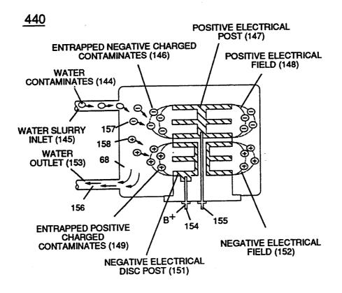
FIGURE 3-45: ELECTROSTATIC FILTER ASS'Y
