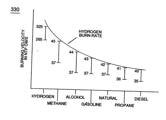
FIGURE 3-37: HYDROGEN BURN-RATE
